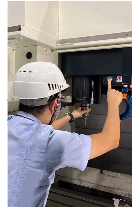
Easy Spindle accessibility for tool loading at spindle side
