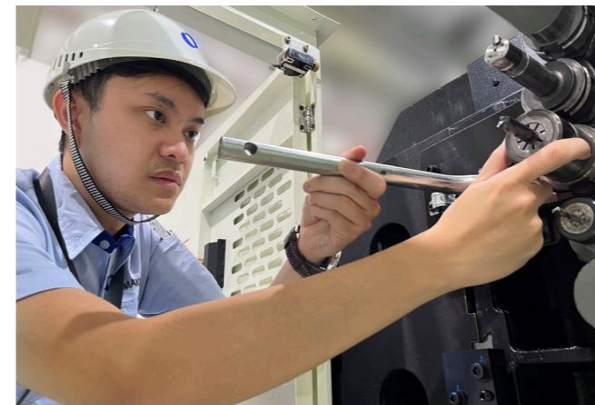
Easy ATC magazine accessibility for tool loading at magazine side
