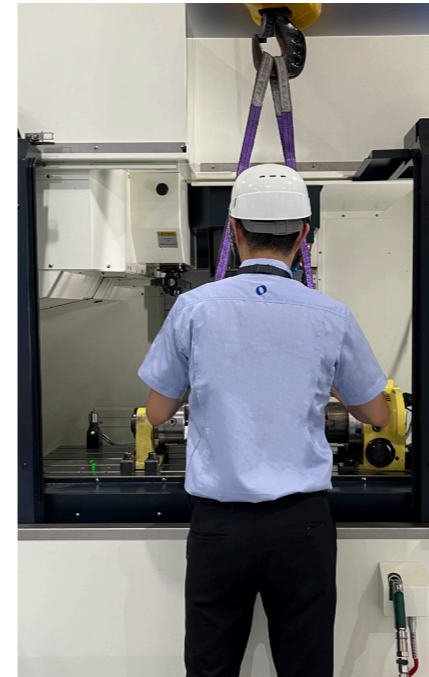
The machine ceiling opens, to facilitate easy handling of large, heavy workpieces and fixtures that require an overhead crane
