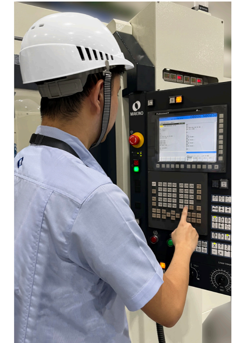
Easy operation with good hand eye coordination aided by 90° swing of operation panel
