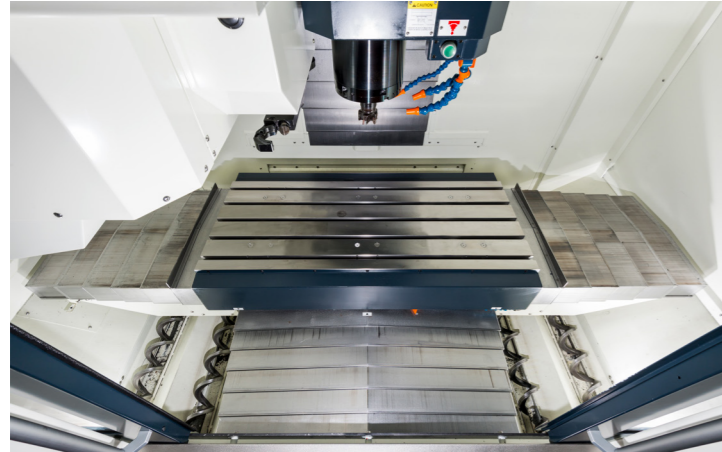
*Picture of PS105 with two spiral conveyors on each side *PS65 comes with one spiral conveyor on each side
