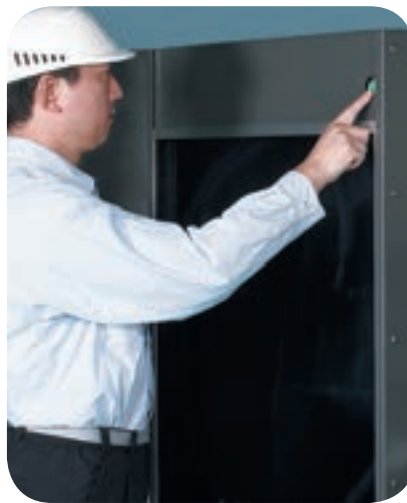
Air is blown by pressing the button and evacuates water captured inside the filter.
