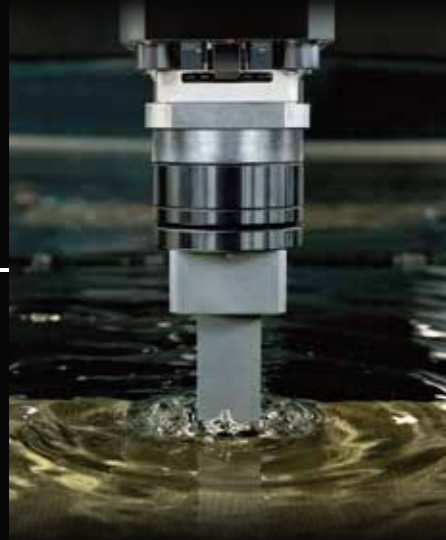
EDM machines can contribute to dies/molds production especially in machining thin and deep shape.
